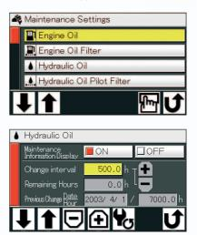
Replacement timing of hydraulic oil and fuel filters is alerted to the operator through the LCD monitor according to the schedule preset by the user each time when turning the key switch. The scheduled maintenance can prevent the failure of the machine. Attachement support system (work mode selector)
