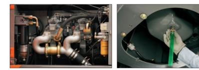
Wide doors give access, from ground level, to the fuel filter, water separator and engine oil filter. A large handrail, steps and anti-skid plates lead to the engine cover. The engine oil pan is fitted with a drain coupler. When draining, an associated drain hose is connected to the drain coupler. The drain coupler is reliable, avoiding oil leakage and vandalism.
