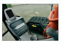
The color LCD monitor, located in the cab, indicates coolant temperature, fuel level, and maintenance data. It also allows one-touch adjustment of the attachment. The display can also be adjusted to day or night shift.
