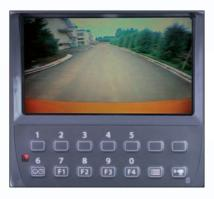
The widescreen color LCD, teamed up with the rear view camera on the counterweight, gives the operator unobstructed rearward viewing. The rear view camera automatically works when traveling, and can also be manually turned on with a select switch on the monitor.
